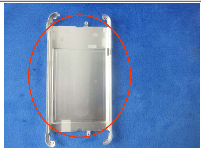
WIFI/BT/BLE/GPS – Metallic Antenna View
