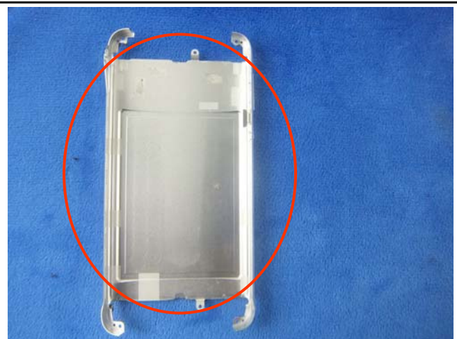
WIFI/BT/BLE/GPS – Metallic Antenna View
