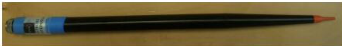
Figure 1 – MVG COMOSAR Dosimetric E field Dipole
