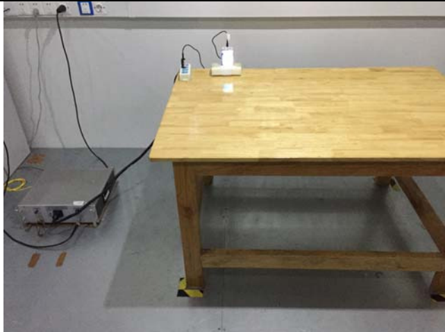
Conducted Emissions Test Setup Front View
