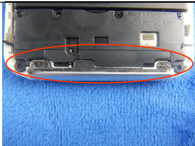
GSM/PCS/UMTS-FDD Antenna View
