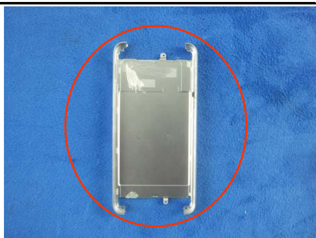
WIFI/BT/BLE/GPS – Metallic Antenna View
