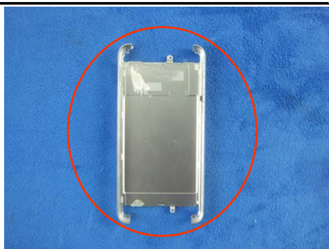
WIFI/BT/BLE/GPS – Metallic Antenna View
