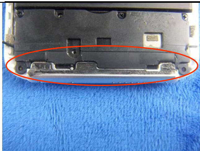
GSM/PCS/UMTS-FDD Antenna View
