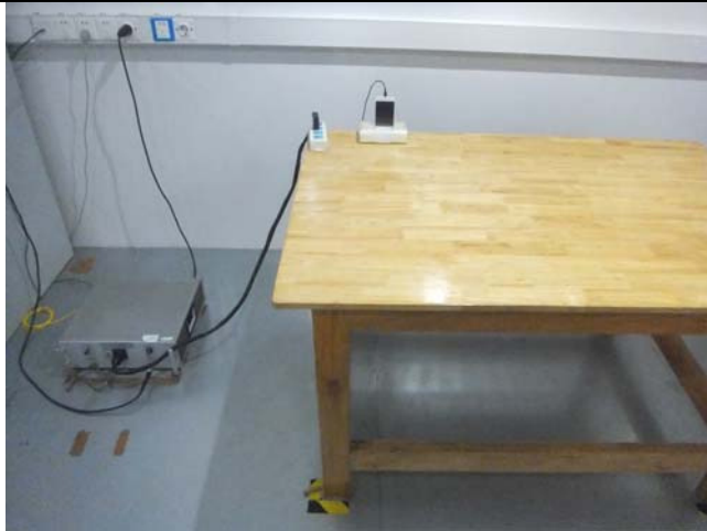
Conducted Emissions Test Setup Front View
