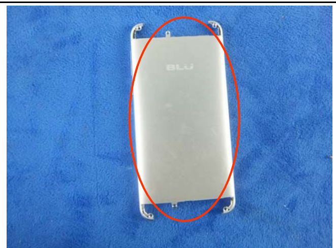
WIFI/BT/BLE/GPS – Metallic Antenna View
