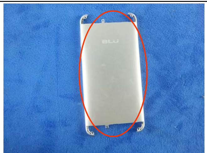
WIFI/BT/BLE/GPS – Metallic Antenna View
