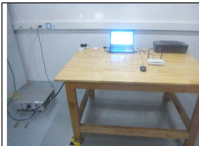
Conducted Emissions Test Setup – Front View
