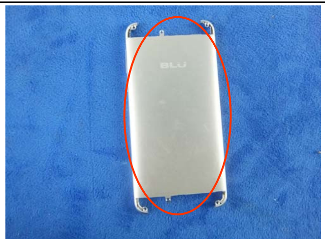
WIFI/BT/BLE/GPS – Metallic Antenna View
