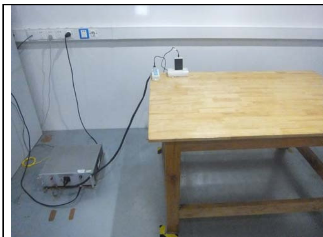
Conducted Emissions Test Setup Front View
