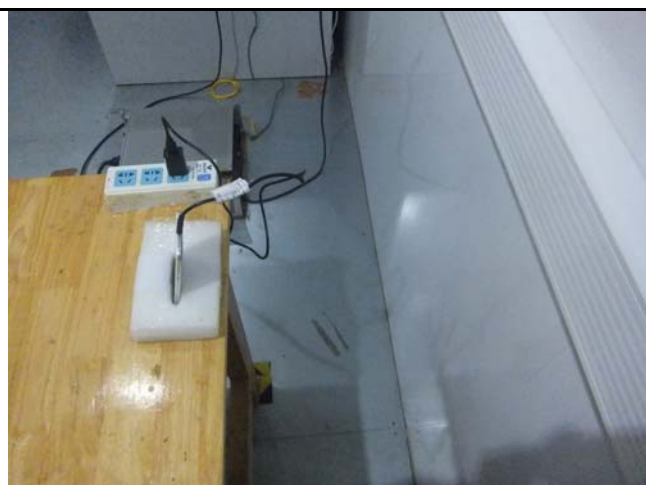
Conducted Emissions Test Setup Side View
