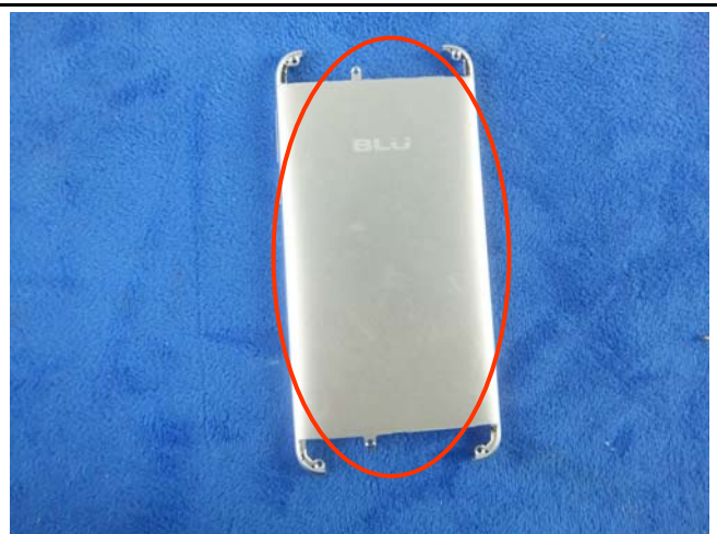
WIFI/BT/BLE/GPS – Metallic Antenna View
