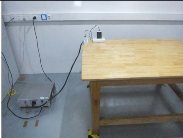
Conducted Emissions Test Setup Front View
