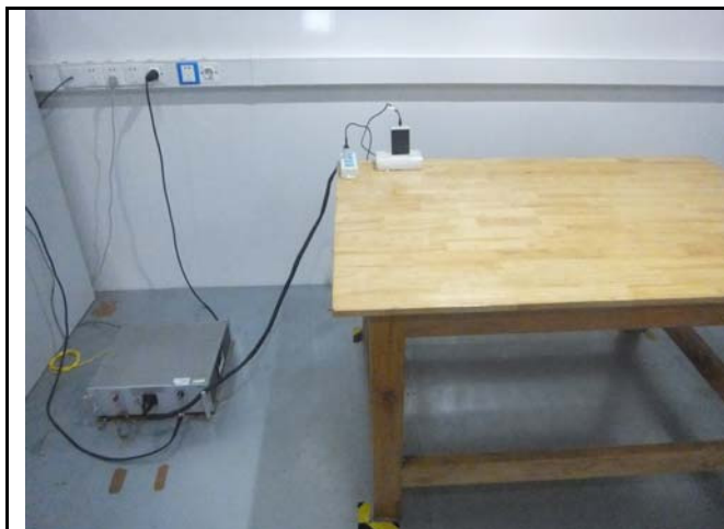
Conducted Emissions Test Setup Front View
