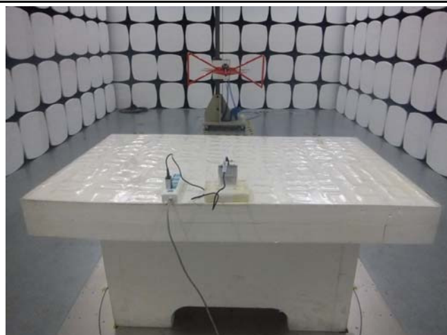
Conducted Emissions Test Setup Front View
