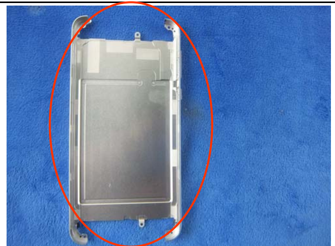
WIFI/BT/BLE/GPS – Metallic Antenna View
