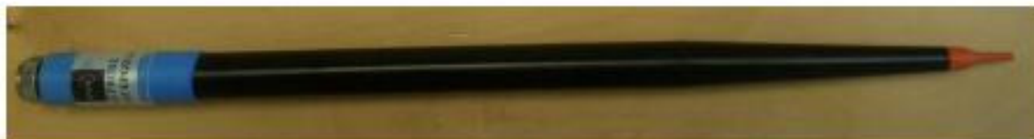
Figure 1 – MVG COMOSAR Dosimetric E field Dipole
