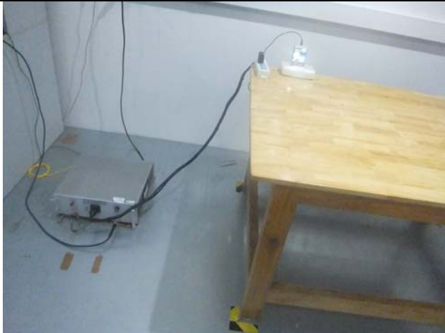
Conducted Emissions Test Setup Front View
