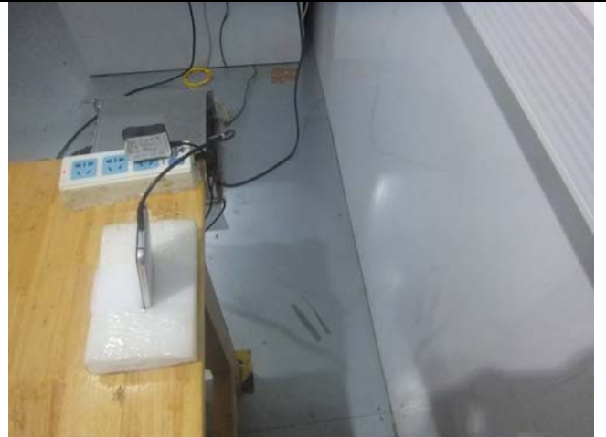
Conducted Emissions Test Setup Side View
