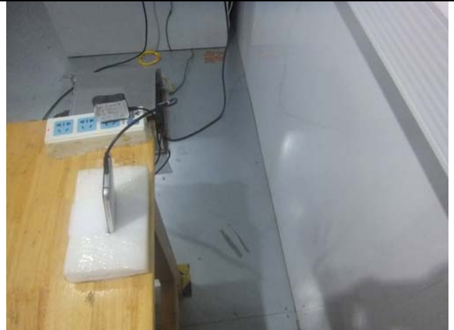
Conducted Emissions Test Setup Side View
