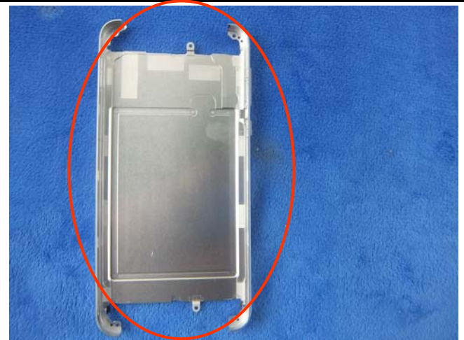
WIFI/BT/BLE/GPS – Metallic Antenna View
