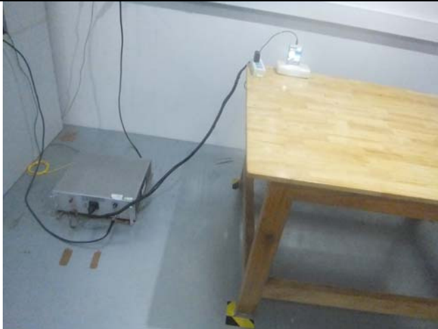
Conducted Emissions Test Setup Front View
