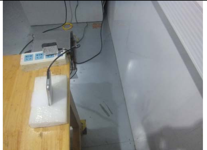
Conducted Emissions Test Setup Side View
