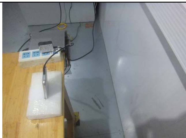
Conducted Emissions Test Setup Side View
