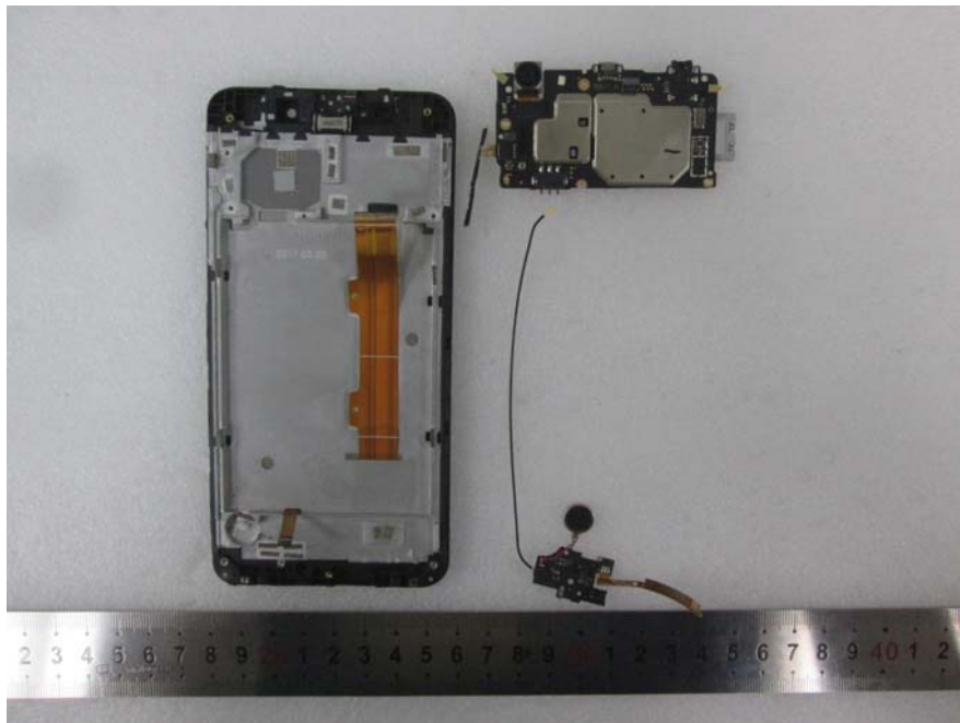
EUT – Cover off View 3
