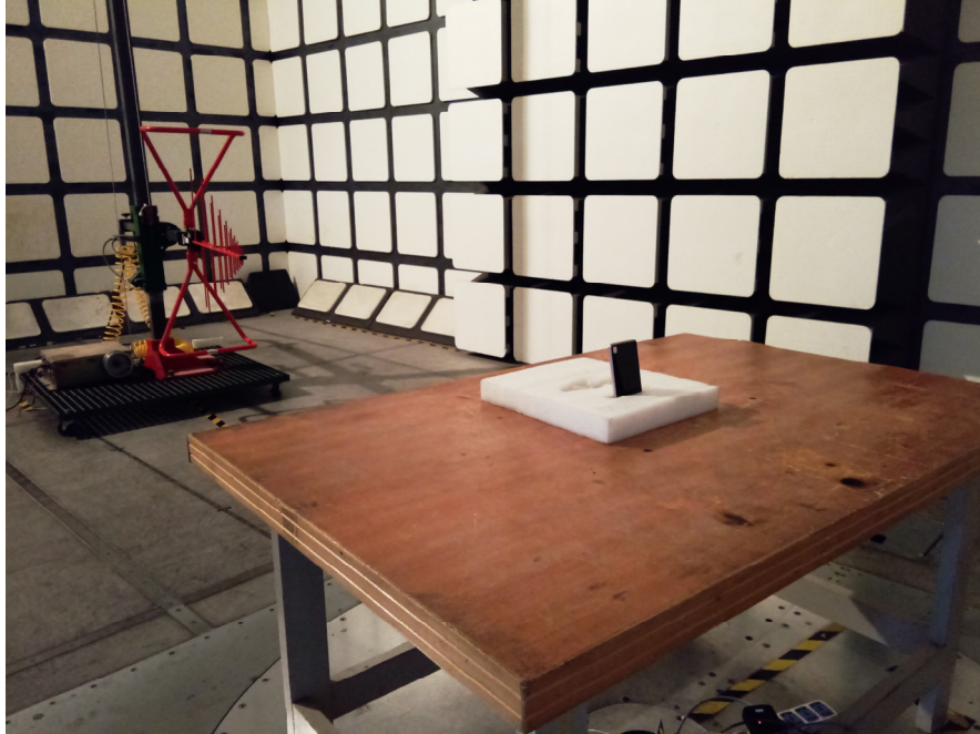
Radiated Emissions View (Below 1 GHz)
