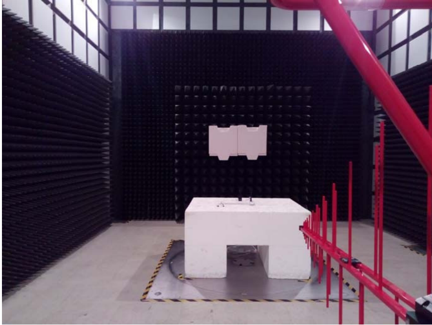
Radiated Emissions View (Below 1 GHz)
