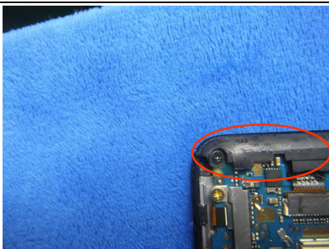
LTE - Antenna View
