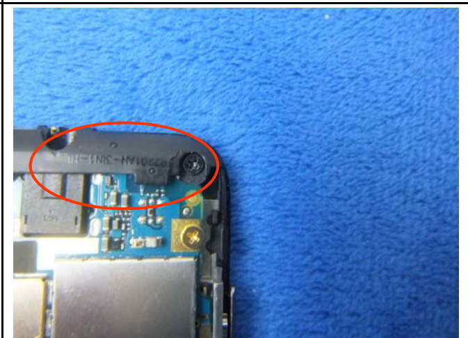
WIFI/BT/BLE/GPS - Antenna View
