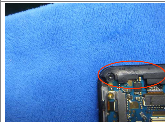
LTE - Antenna View
