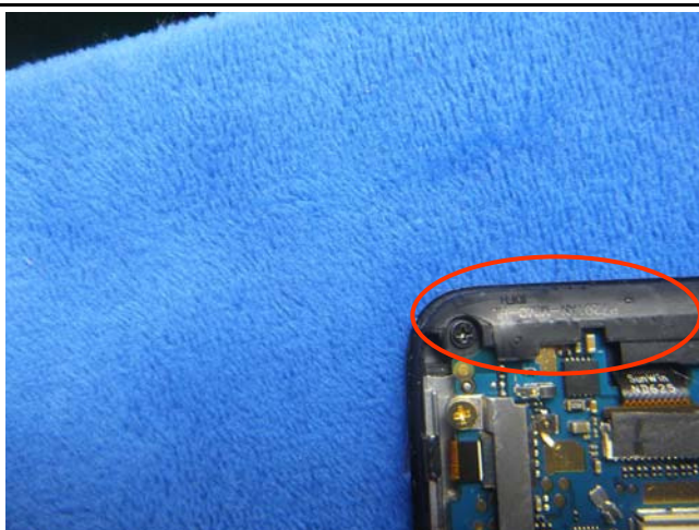
LTE - Antenna View
