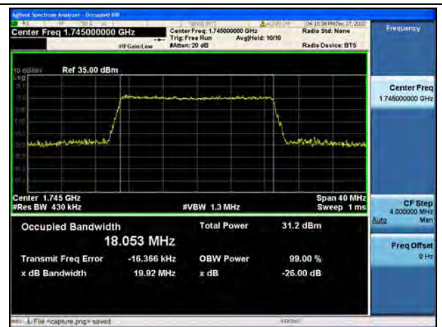
Band66 / 20MHz / 16QAM/ Mid CH
