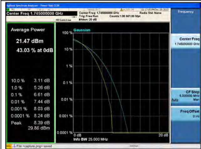
Band66 / 20MHz / Mid CH / 64QAM
