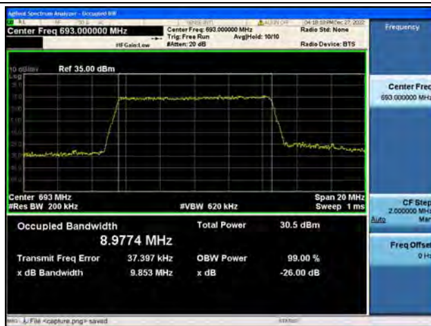
Band71 / 10MHz / 16QAM/ High CH
