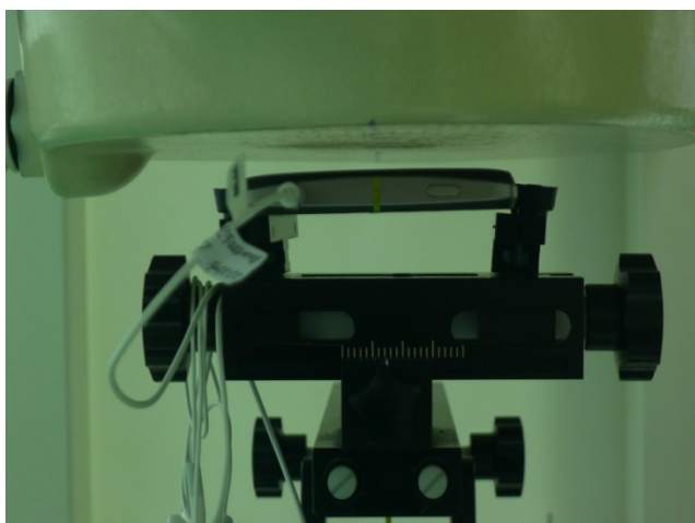
Back Side of the DUT with Phantom 1 cm Gap (with Headset)
