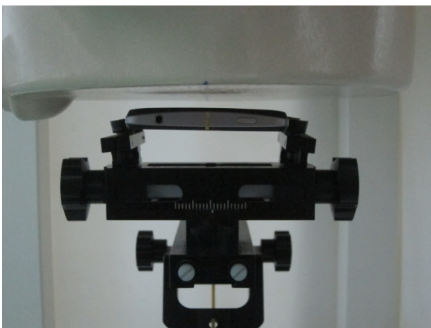
Back Side of the DUT with Phantom 1 cm Gap
