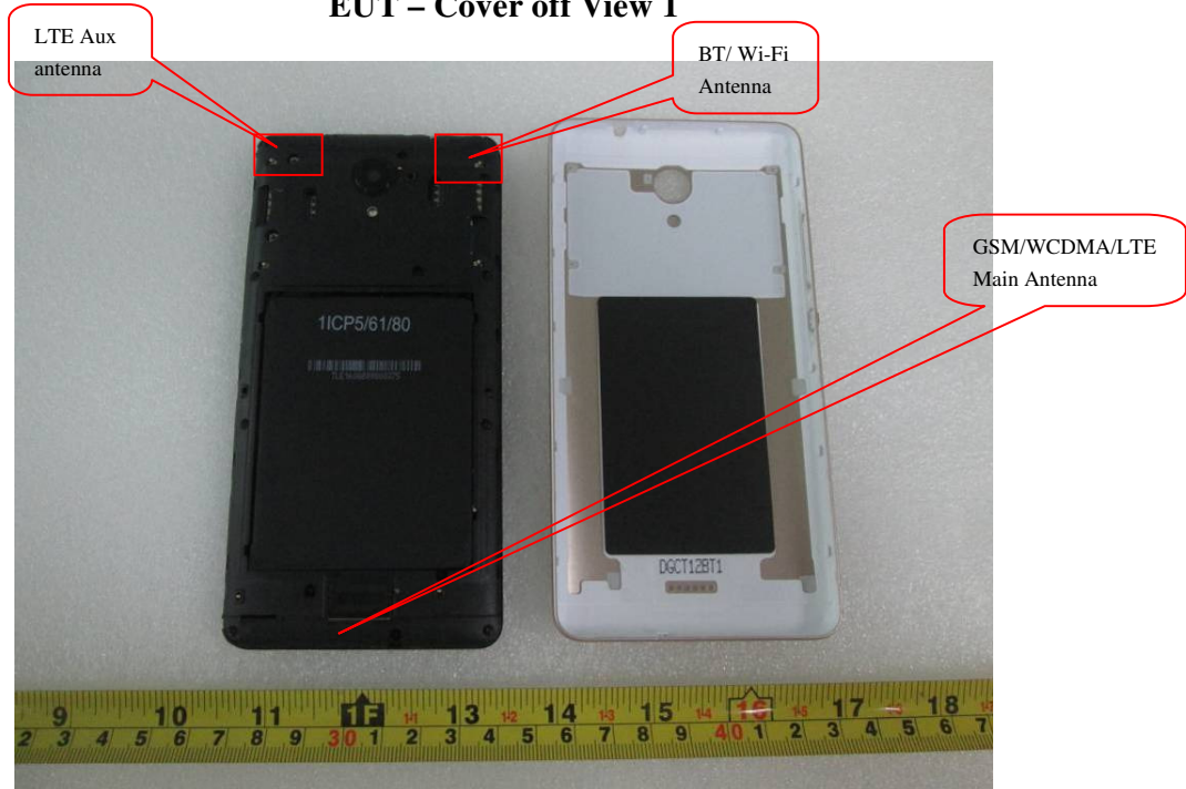
EUT – Cover off View 1
