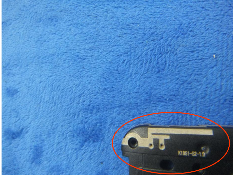
LTE - Antenna View
