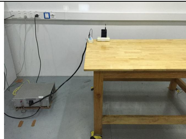
Conducted Emissions Test Setup Front View
