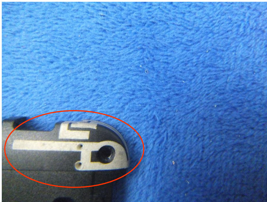
BT/WIFI - Antenna View
