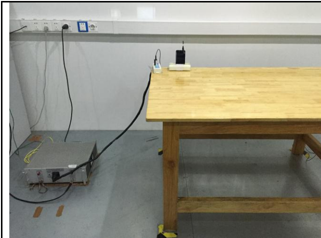
Conducted Emissions Test Setup Front View
