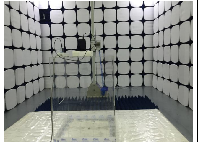
Radiated Spurious Emissions Test Setup Above 1GHz
