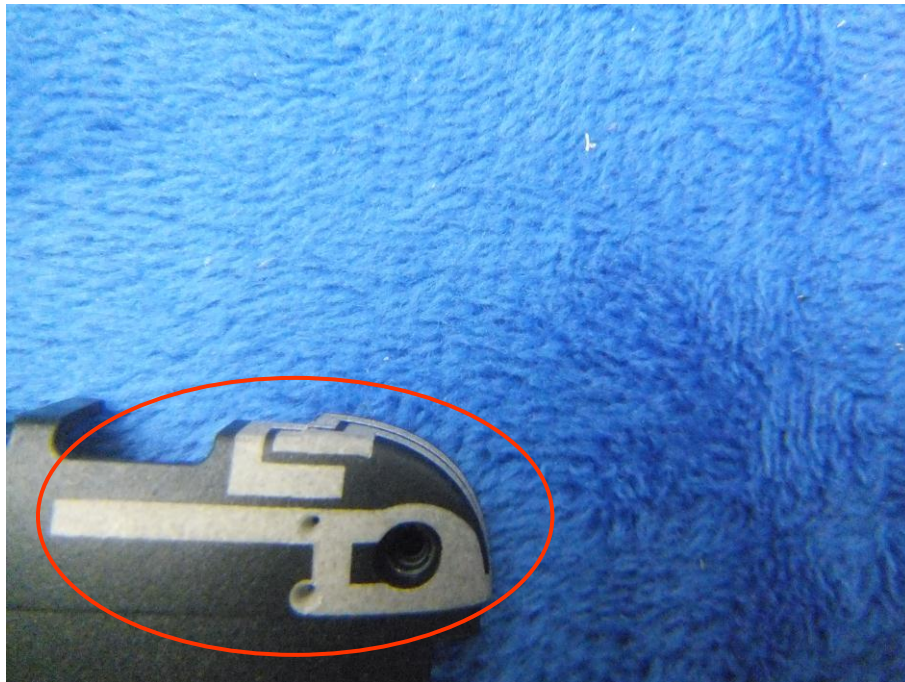
BT/WIFI - Antenna View
