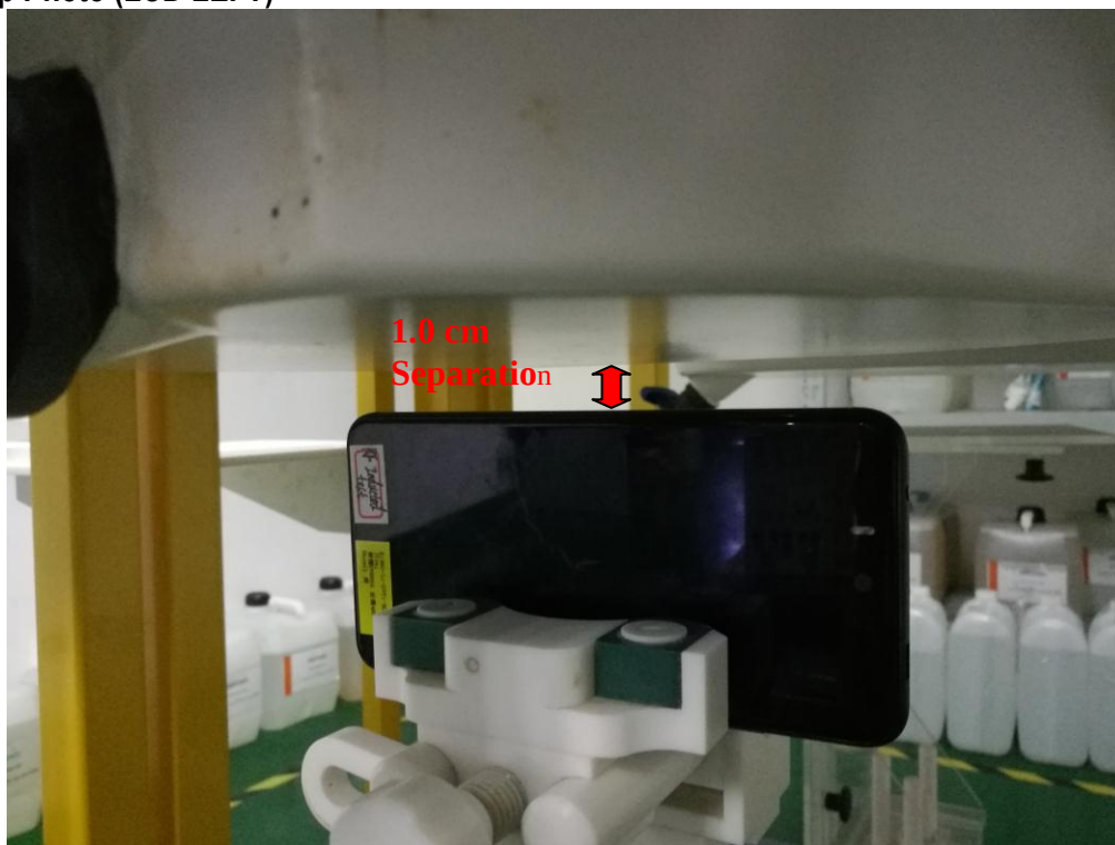
Body Setup Photo (LCD RIGHT)
