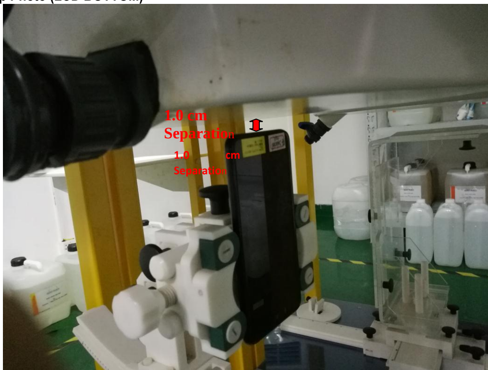
Body Setup Photo (LCD BOTTOM)
