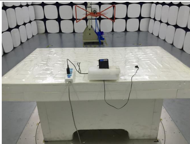
Conducted Emissions Test Setup Front View
