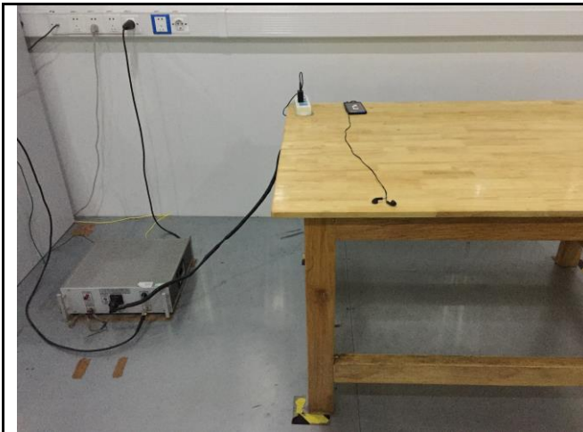
Conducted Emissions Test Setup Front View
