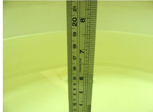
Fig 6.2 Photo of Liquid Height for Body SAR
