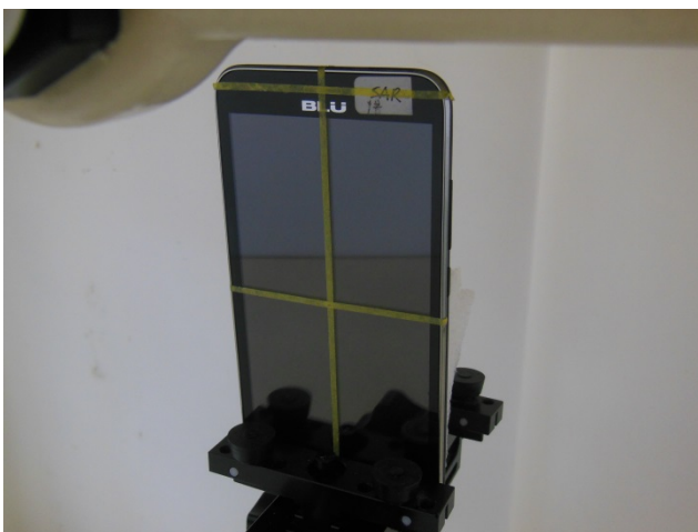
Top Side, Test Separation 1 cm
