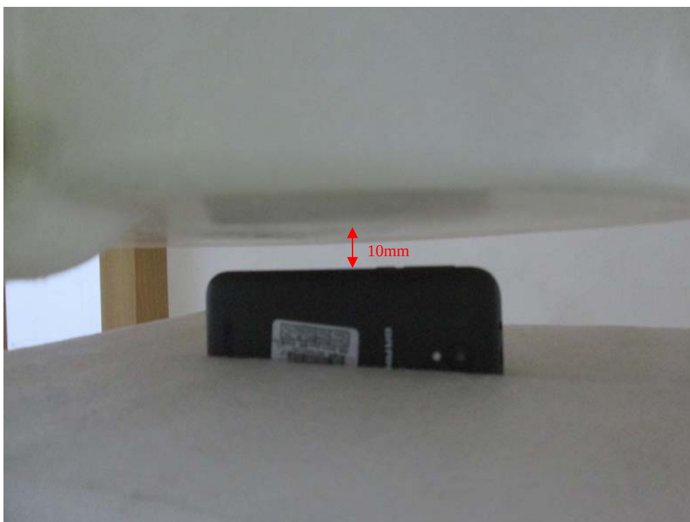
Body-worn Right Setup Photo (10mm)
