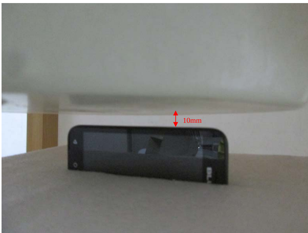
Body-worn Left Setup Photo (10mm)
