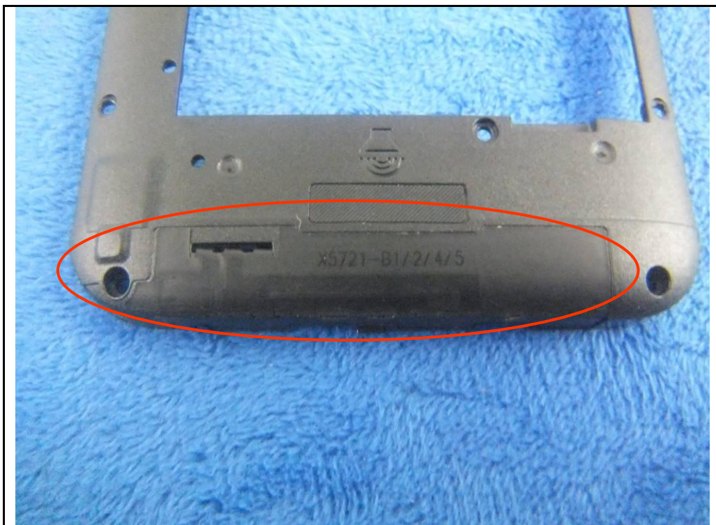
GSM/PCS/UMTS-FDD Antenna View
