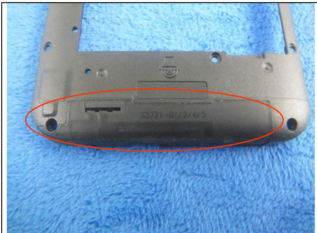
GSM/PCS/UMTS-FDD Antenna View
