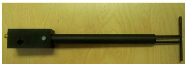
Figure 1 – MVG COMOSAR Validation Dipole
