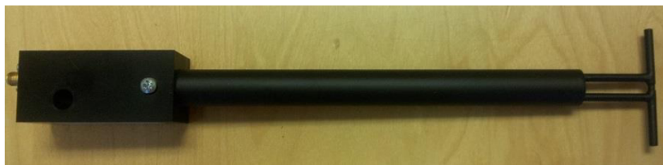
Figure 1 – MVG COMOSAR Validation Dipole
