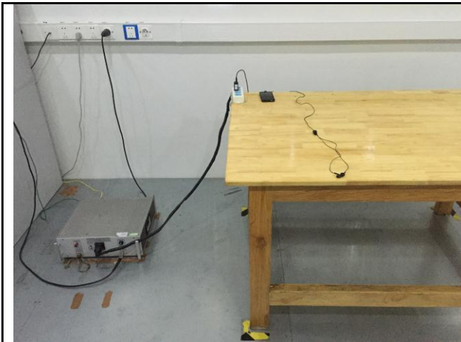
Conducted Emissions Test Setup Front View
