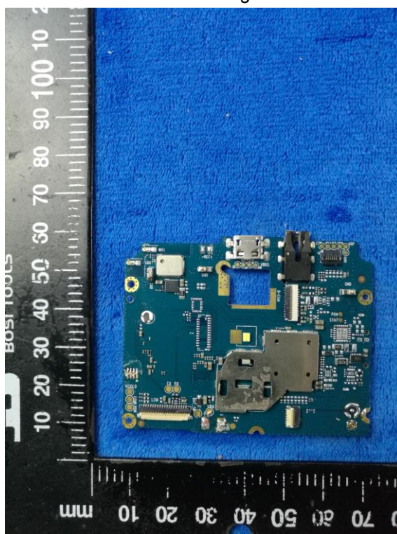
Mainboard with Shielding – Rear View
