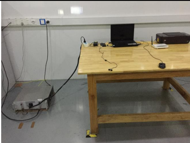
Conducted Emissions Test Setup – Front View
