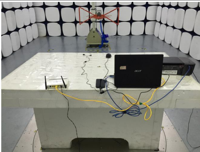
Radiated Emissions Test Setup Below 1GHz
