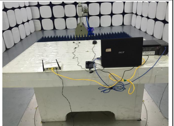
Radiated Emissions Test Setup Above 1GHz
