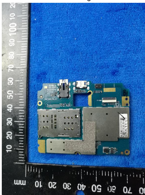
Mainboard with Shielding – Front View
