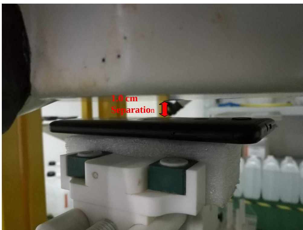
Body Setup Photo (LCD DOWN)
