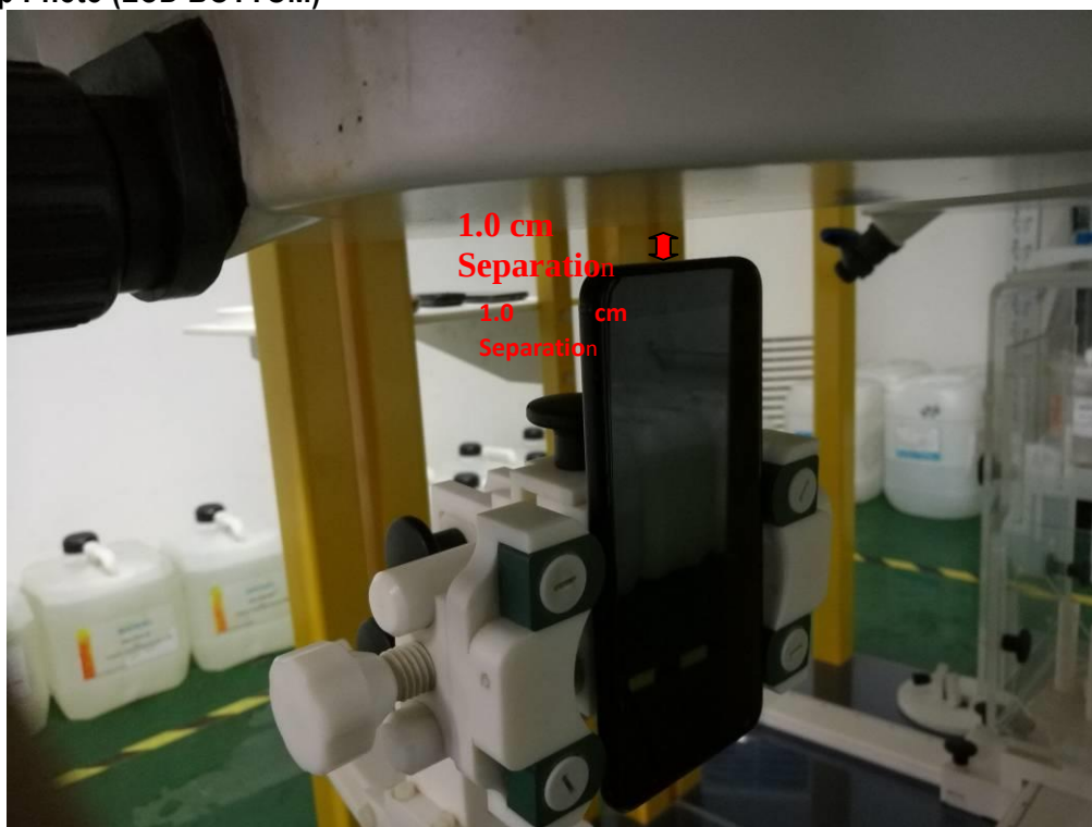
Body Setup Photo (LCD BOTTOM)
