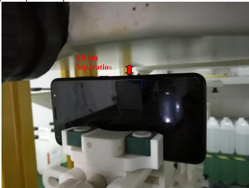
Body Setup Photo (LCD RIGHT)
