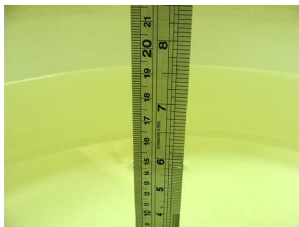
Fig 6.2 Photo of Liquid Height for Body SAR
