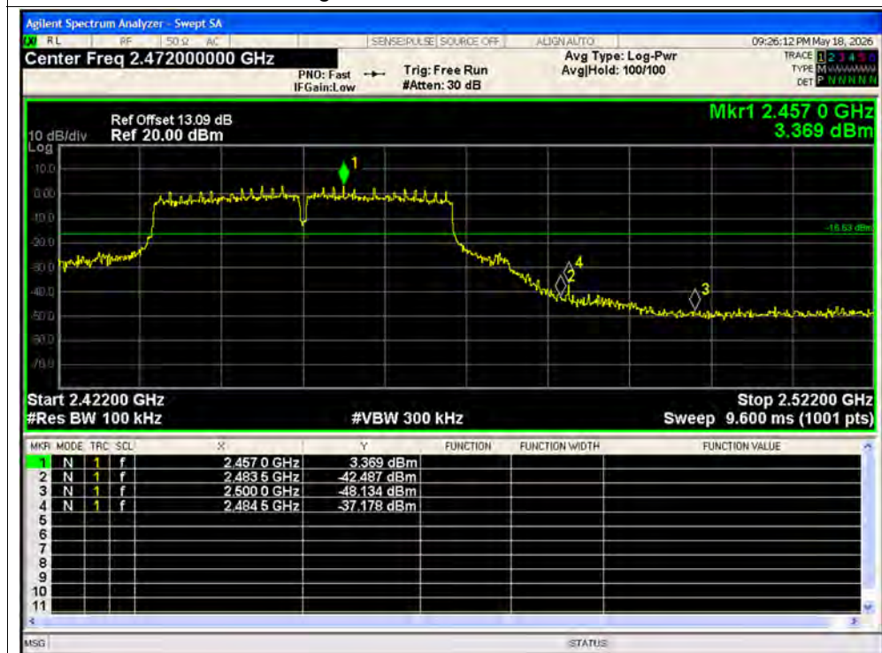
Band Edge NVNT ac40 2452MHz Ant1 Emission
