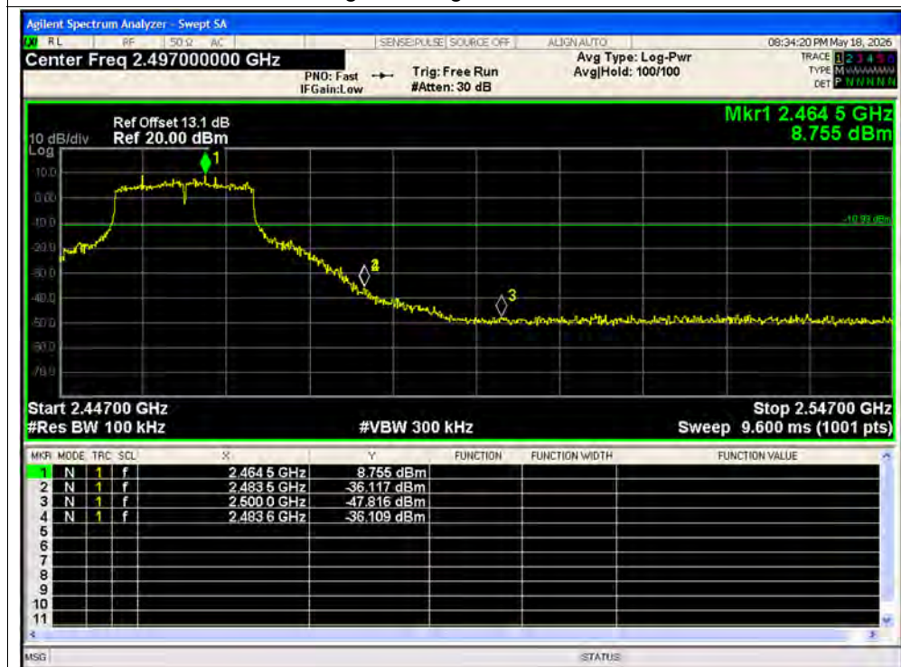
Band Edge NVNT g 2462MHz Ant1 Emission
