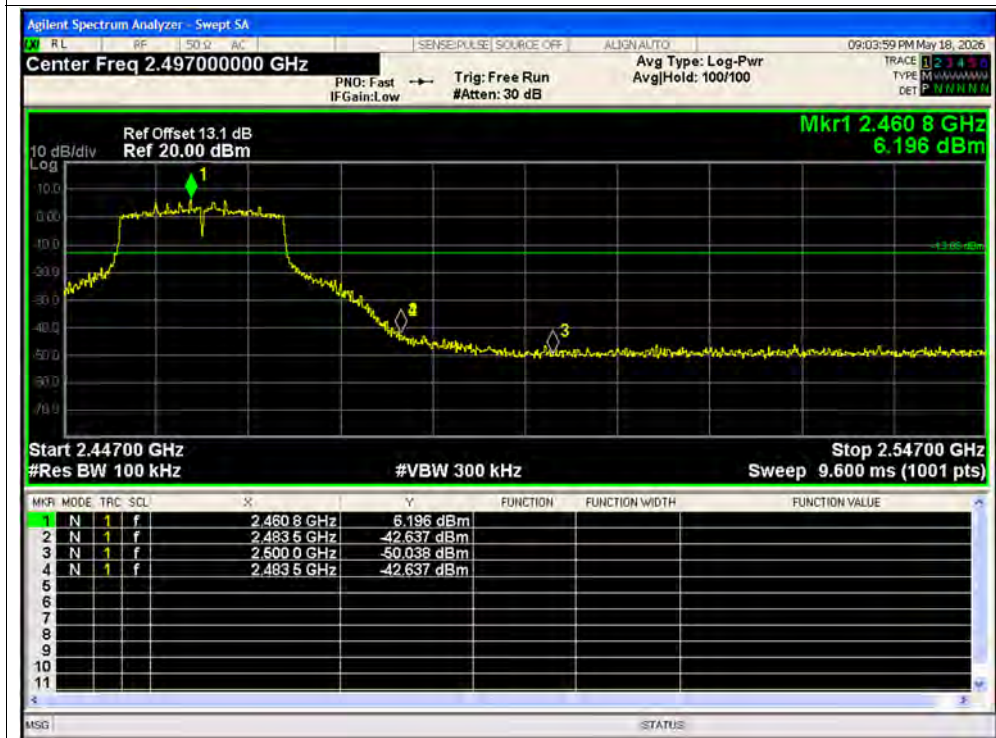
Band Edge NVNT ac20 2462MHz Ant1 Emission
