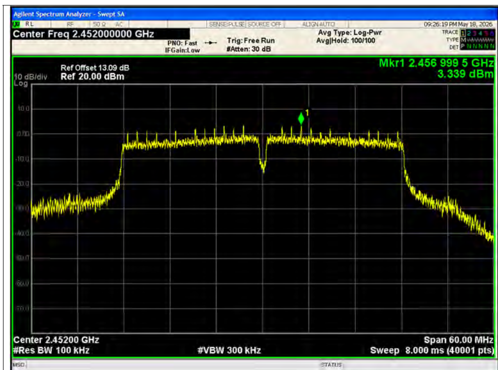
Tx. Spurious NVNT ac40 2452MHz Ant1 Ref
