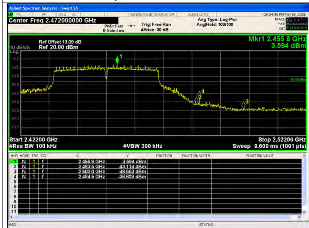
Band Edge NVNT n40 2452MHz Ant1 Emission
