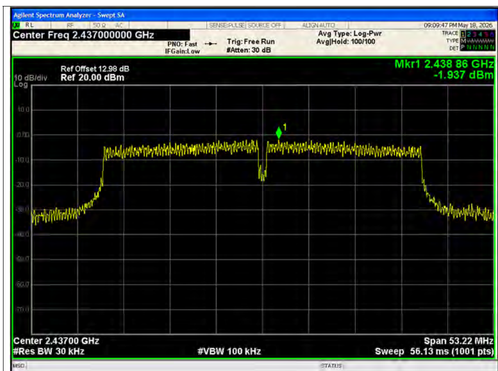
PSD NVNT ac40 2437MHz Ant1
