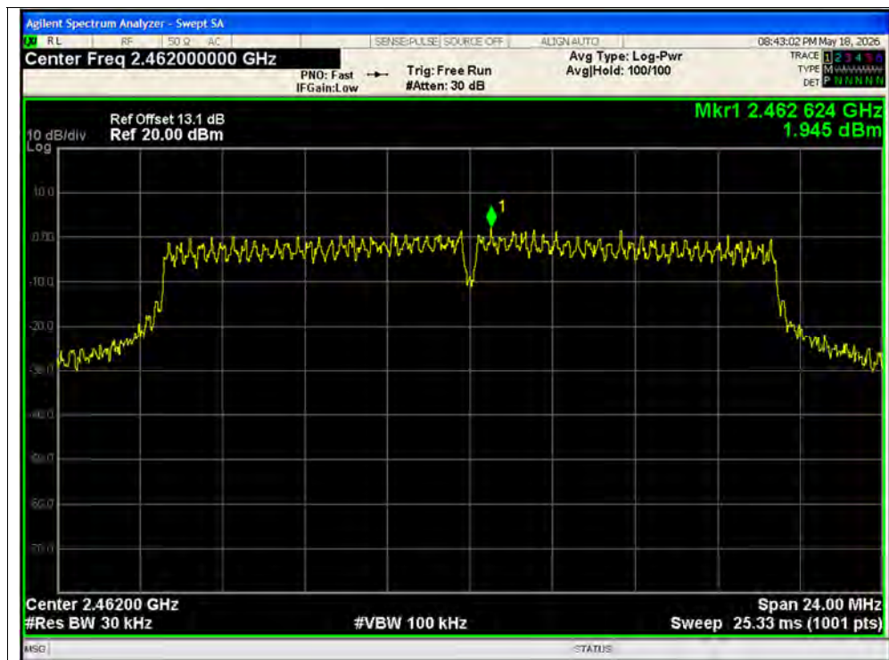
PSD NVNT n20 2462MHz Ant1
