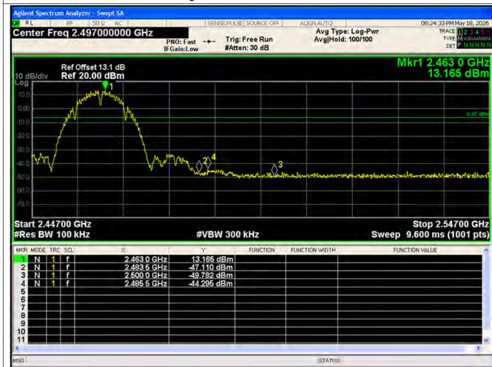
Band Edge NVNT b 2462MHz Ant1 Emission
