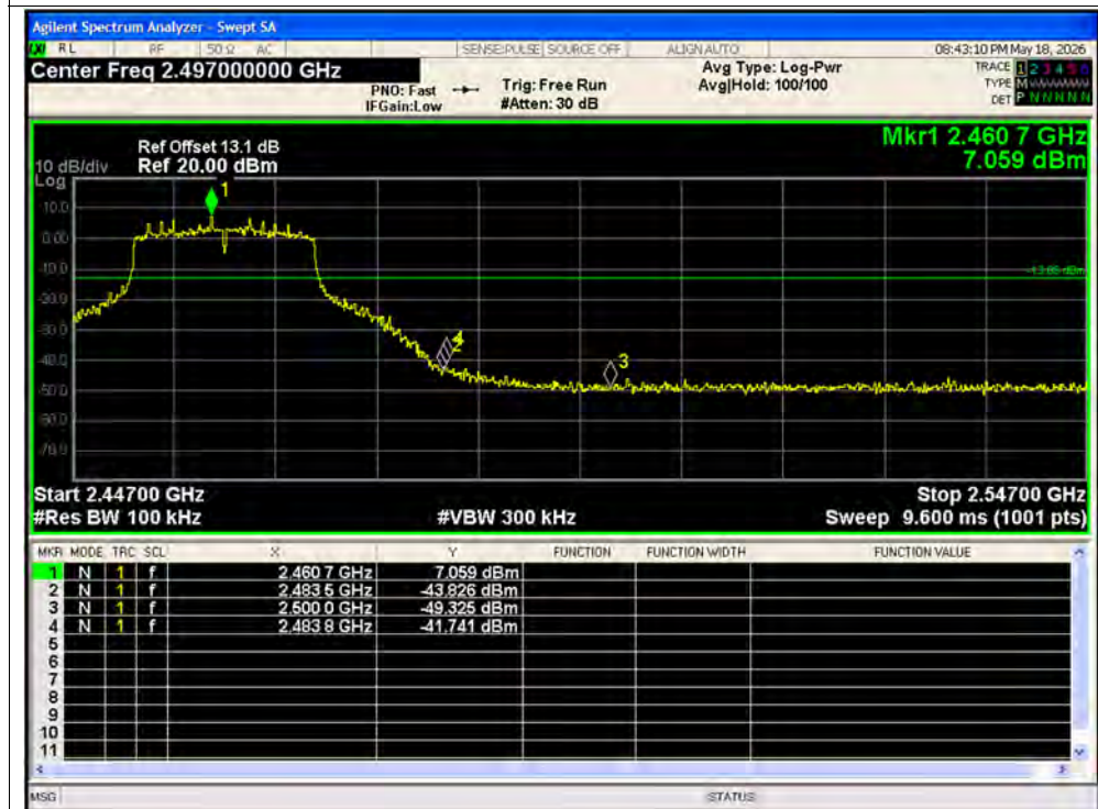
Band Edge NVNT n20 2462MHz Ant1 Emission
