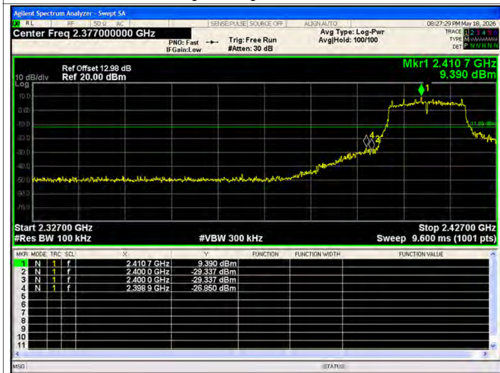
Band Edge NVNT g 2412MHz Ant1 Emission
