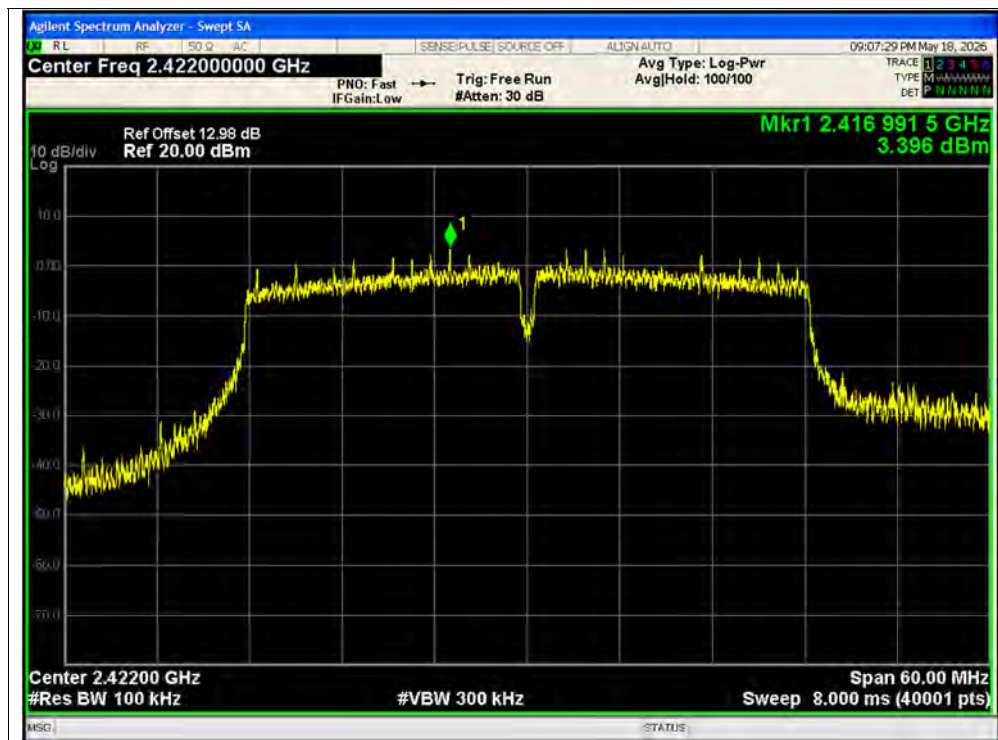
Tx. Spurious NVNT ac40 2422MHz Ant1 Ref
