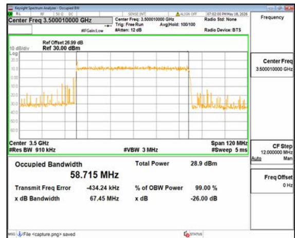
n77(3450-3550MHz) 60M DFT-s-OFDM QPSK Outer_Full Mid
