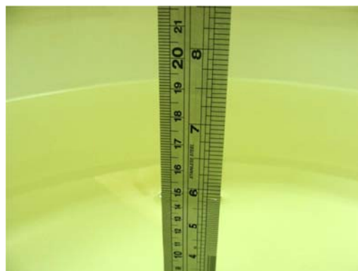
Fig 6.2 Photo of Liquid Height for Body SAR
